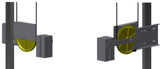
The rope must have enough tension. In the event of tension loosening a rope slackening contact (1) connected to the installation security series will cut off the current.
