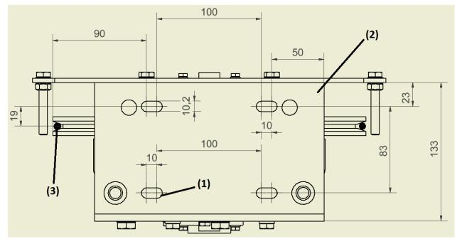
The above figure represents the bottom view of the governor base plate (2).
