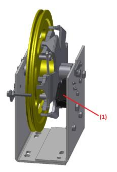
The governor has a built-in overspeed contact.
