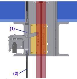
The tension weight is secured to the guide rail by flanges.
