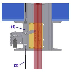
The tension weight is secured to the guide rail by flanges.
