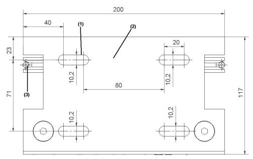
The above figure represents the bottom view of the governor base plate (2).
