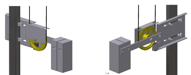
The rope must have enough tension. In the event of tension loosening a rope slackening contact (1) connected to the installation security series will cut off the current.
