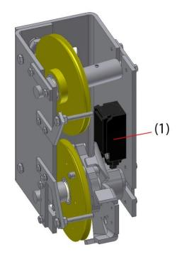
Once the governor and, therefore, the safety gear have been interlocked, when unjamming the safety gears, the return spring will return to its initial resting position and, therefore, the overspeed contact will reset on its own.
